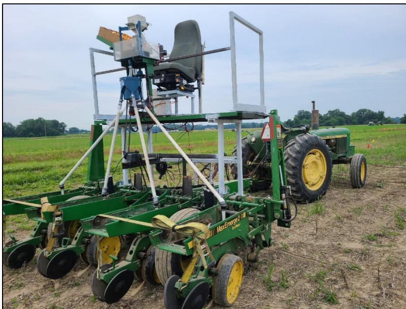
Figure 1. Modified no-till planter fabricated in 2021 for no-till planting of all plots in the test.
